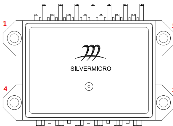
Fig 9 The module with 4 mounting holes
